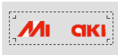
1. Detect register marks and cut outside of the marks.
