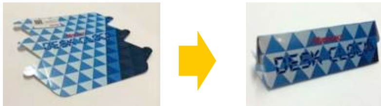
Creasing make it easy for folding the packaging
