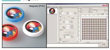
Total printing time (White printing+Color printing): 22 min., 24 sec. Size: 29 mm dia., 1,200 x 1,200 dpi, 16 pass Hi-mode Width 600 mm x feeding direction 500 mm, with 168 units imposed.
