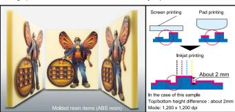
Note:To prevent the occurrence of problems due to ink mist when printing on three-dimensional items, the area around the head should be cleaned frequently. Also, the greater the distance from the head, the more the printing guality declines, so prior testing is necessary.
